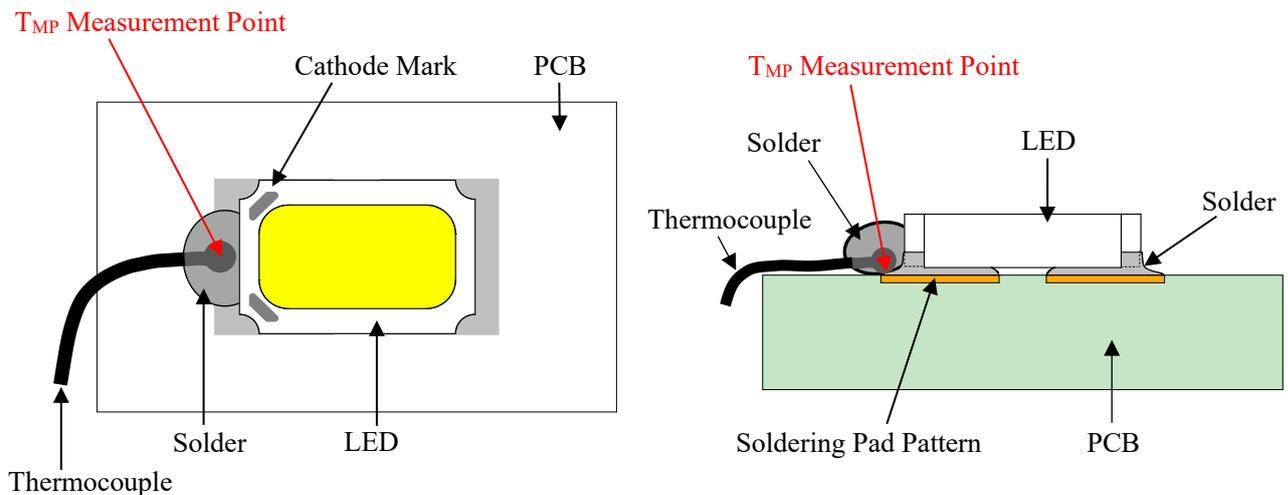
Figure 2.  $T_{MP}$  Measurement Point
