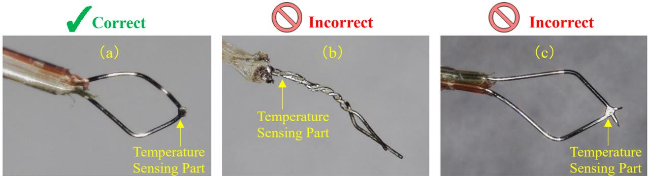
Figure 4. Temperature Sensing Part of Thermocouples
