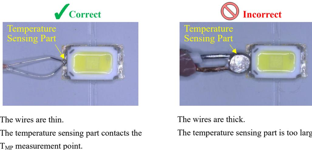
Figure 3. Examples of Correct/Incorrect Thermocouples
