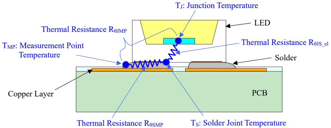
Figure 1. Cross-sectional View of the LED Mounted on a PCB and a Simple Thermal Resistance Model
